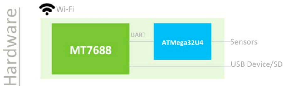
Figure 44 LinkIt Smart 7688 Duo Hardware Architecture
